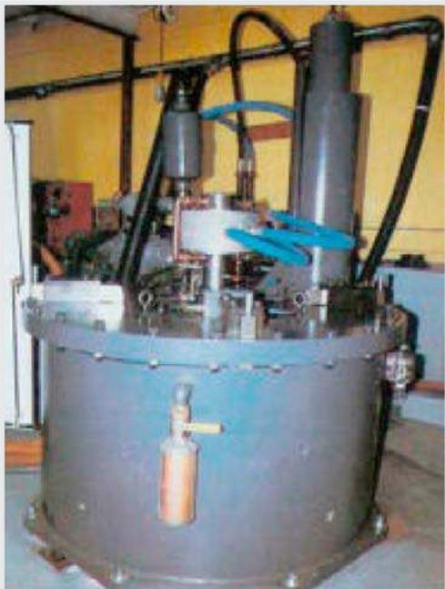
**SPIN TEST SYSTEMS**, which are used extensively in the turbomachinery industry for evaluating the centrifugal strength and fatigue life of high-speed rotating components such as turbine disks and centrifugal compressors, allow stress testing of high-speed components in a controlled environment. Therefore, these systems are faster and less expensive to use than testing in the target engine or machine.
