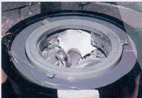
Fig. 3 – To solve the problem, a ledge that would cause the lead to fold back harmlessly into the pit was designed. The model spin pit inside a larger test pit is shown immediately following a lead extrusion containment burst. All the lead was contained inside the pit after the test.
