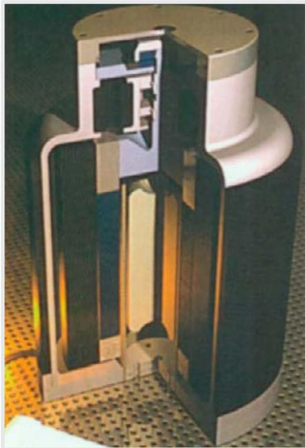
Packed with power that is available on demand, a practical flywheel battery would go a long way toward making low-pollution, high-mileage hybrid electric cars, trucks, and trains a reality. Few other near-term technologies can foreseeably provide the load-leveling (power-averaging) capabilities necessary for rapid acceleration, speed maintenance on grades, and recovery of braking energy (regenerative braking).
