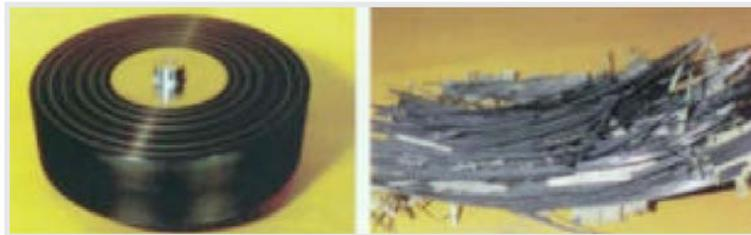
Fig. 4 – Engineers at the Center for Electromechanics fabricated this composite flywheel (left) with weakened graphite fibers so it would burst at a specified rotational speed. Fragments from the wheel failure are shown on the right.
