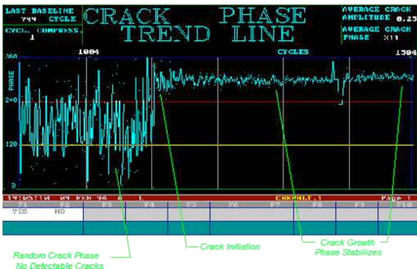
Figure 5 Crack Phase - Bladed Turbine Assembly (cycle range: 24,804 - 25,404)
