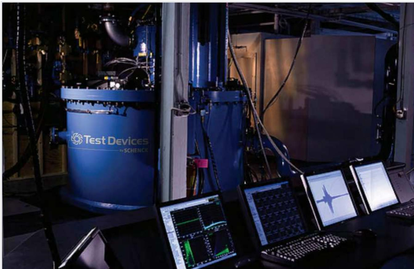
The dynamic spin process was developed in the late 1990s under a U.S. Navy research contract. To make the process more relevant for specific testing applications, the technique was updated and in 2004 Test Devices received a patent addressing both the testing apparatus and method for dynamic resonance testing in a spin rig. Test Devices's patent encompasses a number of items, including a specific nozzle design for the delivery of jet oil as a means of instigating resonant vibratory amplitudes.
