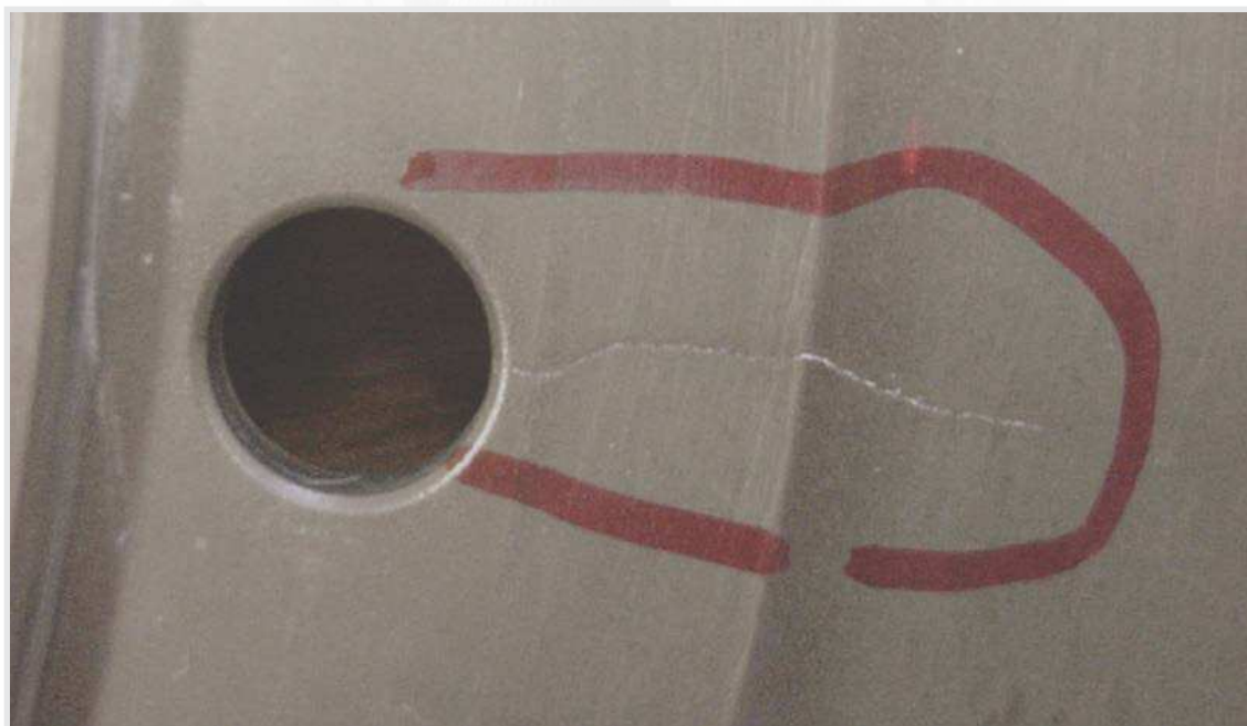
Fig. 1 – Example of a fatigue crack detected before the component failed. The test automatically stopped once the crack was detected.
